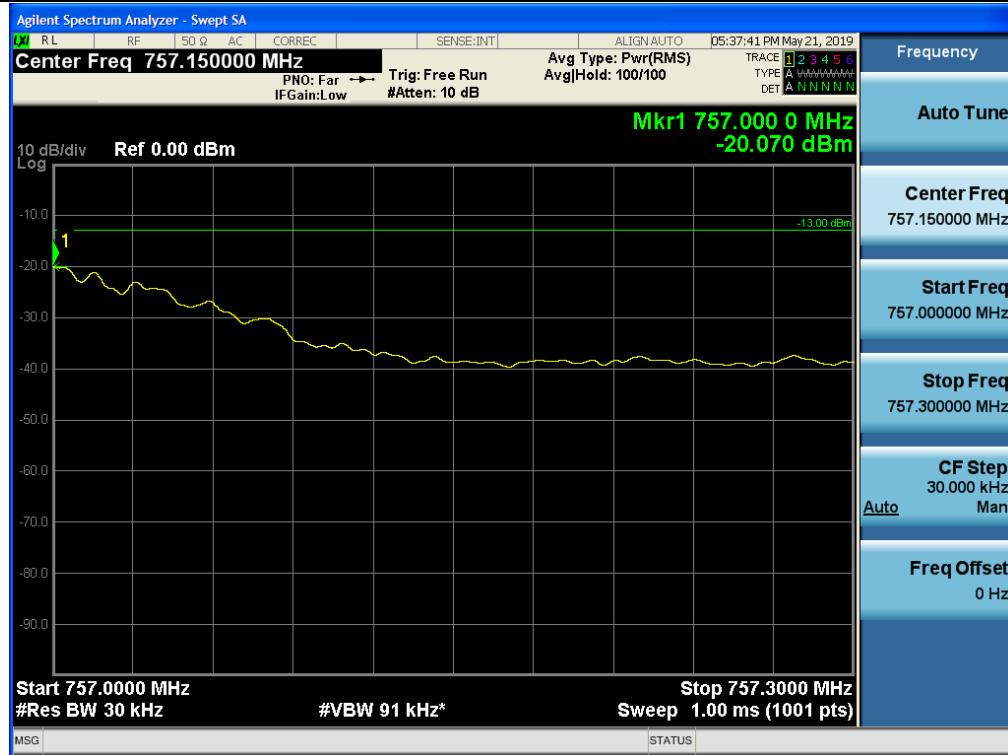
+3 dB above Out-of-band (two adjacent test signals) / Upper 700 MHz / Downlink / LTE 5 MHz / Lower
