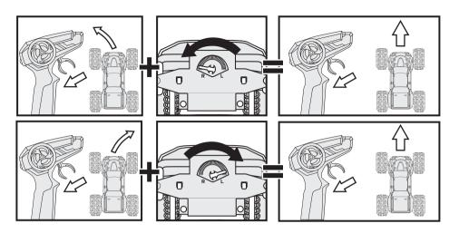
Under your LUMITEK  $RC^{T}$  TERROR TOWER is located a pin that you can turn in order to adjust the wheel alignment if you find out that your truck does not drive straight when not turning the wheel. Check the diagrams above to find out how to adjust on the right or on the left.
