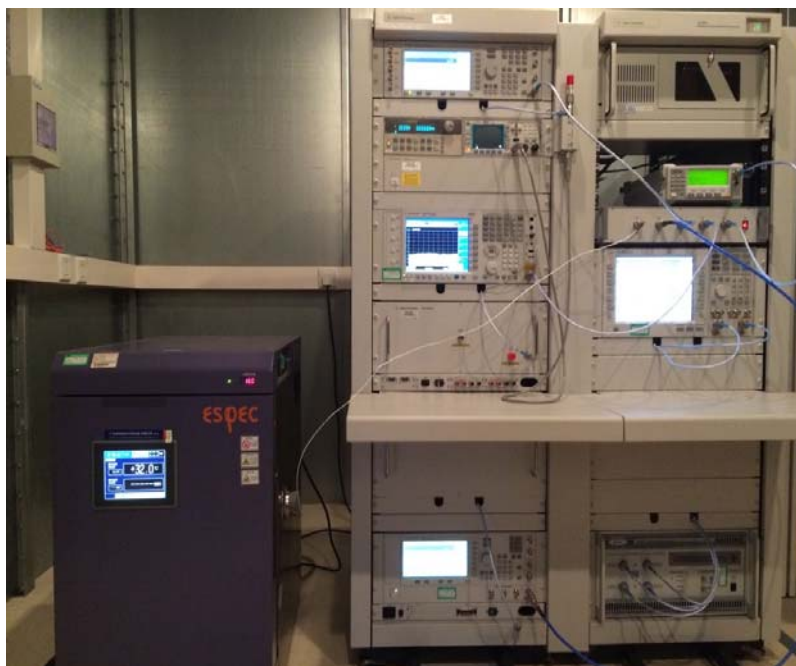
RF setup in extreme condition
