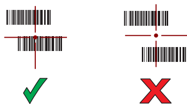
Figure 66 Pick List Mode with Multiple Bar Codes in Aiming Pattern
