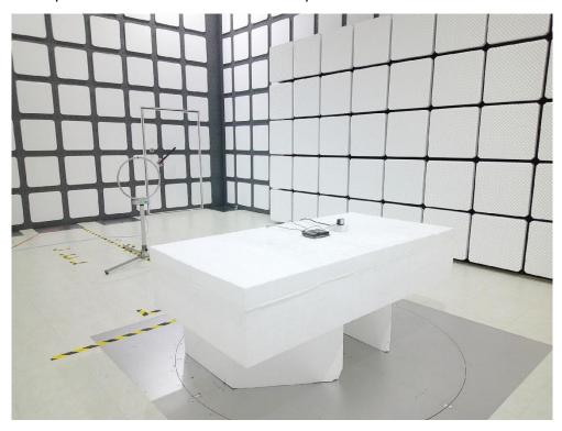
Description: Radiated Emission Test Setup for  $30 \text{MHz} \sim 1 \text{GHz}$
