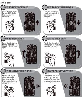
Note: Fine-tuning the steering alignment involves making small adjustments to ensure that the RC car travels straight when the steering control is centered. For example, if the car veers slightly to the left when the control is centered, using the left trim button allows you to correct this deviation, resulting
