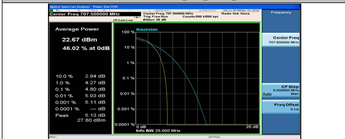
Channel Bandwidth: 10 MHz_MCH_16QAM_1RB#24
