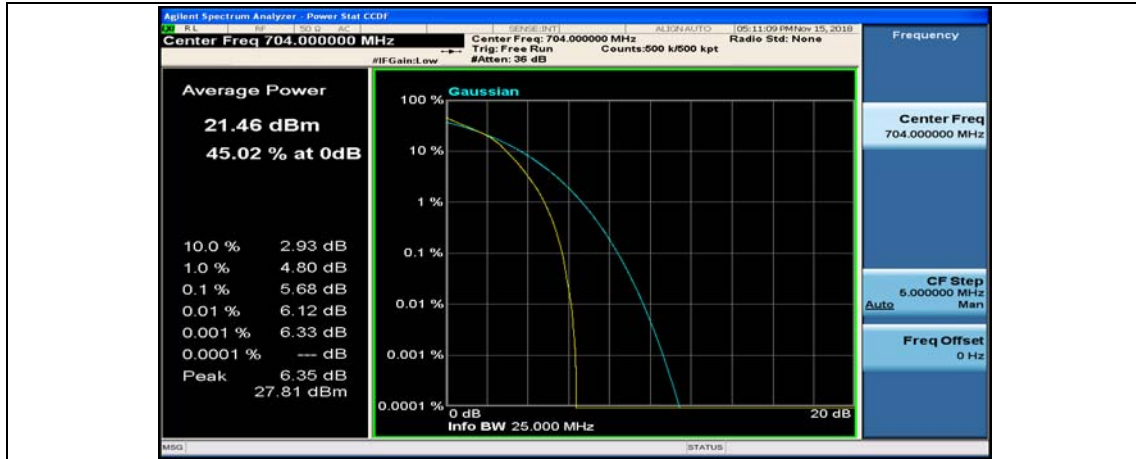
Channel Bandwidth: 10 MHz_MCH_16QAM_1RB#0
