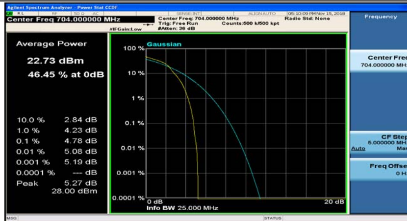
Channel Bandwidth: 10 MHz_LCH_16QAM_1RB#49
