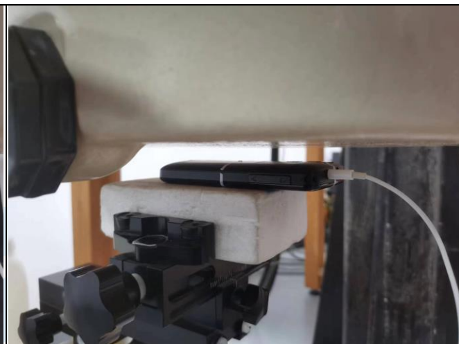
Rear Face of EUT with 1.0 cm Gap ( Headset )
