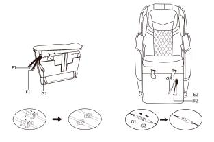
2.Remove the two circlips on the bolts, then attach the footrest onto the base and lock the circlips.
