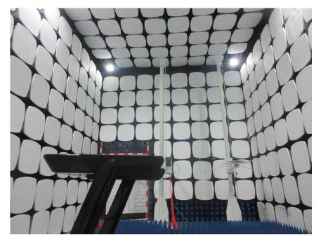
Remark: The transmitter part of the EUT was kept on the high  $1.5 \mathrm{m}$  above  $1 \mathrm{GHz}$  according to the lifting platform during the test.
