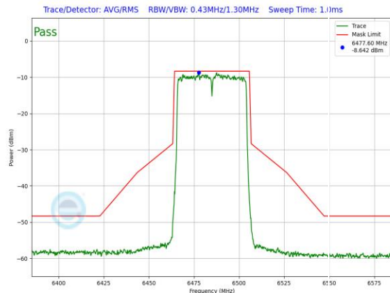
Plot 7-694. LPI In-Band Emission Plot Antenna WF5B (40MHz 802.11ax (UNII Band 6) – Ch. 107, MCS4)
