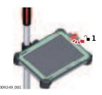
Set the locking lever of the GHT78 holder to the unlocked position.
