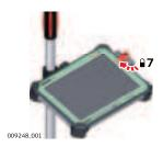
After placing the tablet onto the mounting plate, set the locking lever to the locked position (see illustration).
