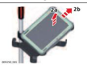
Lift the right side of the tablet and slide the tablet to the right and out of the holder.
