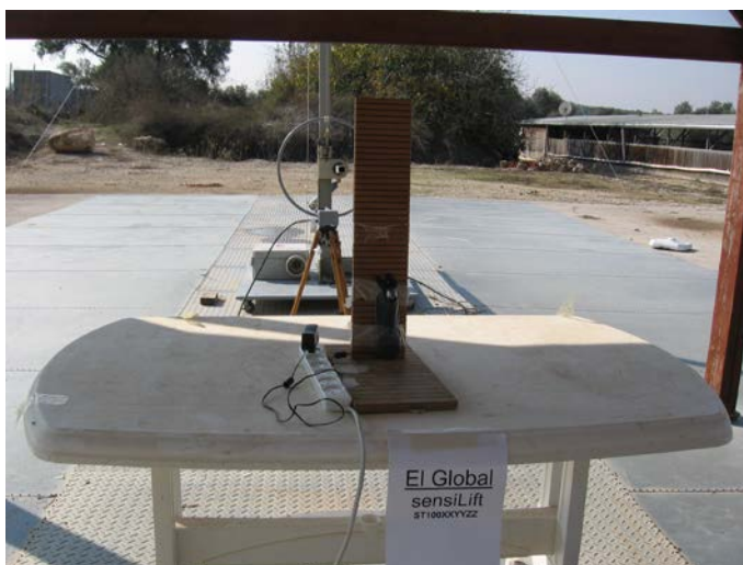
Figure 2. Conducted Emission Test
