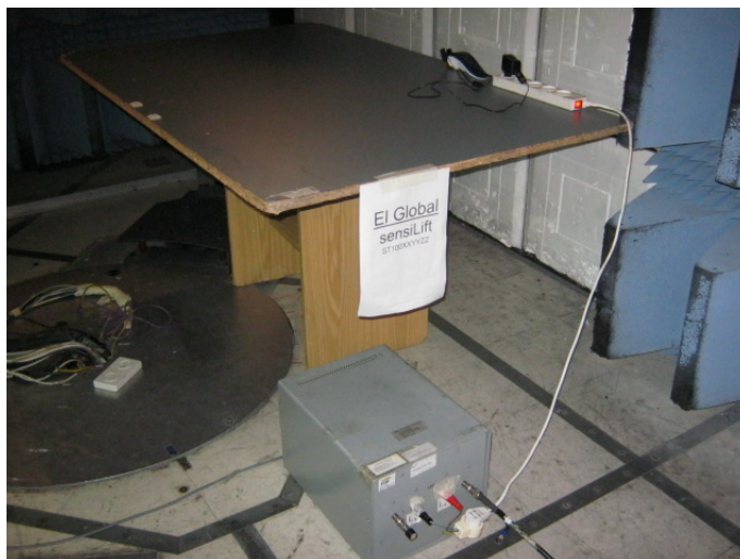
Figure 2. Conducted Emission Test
