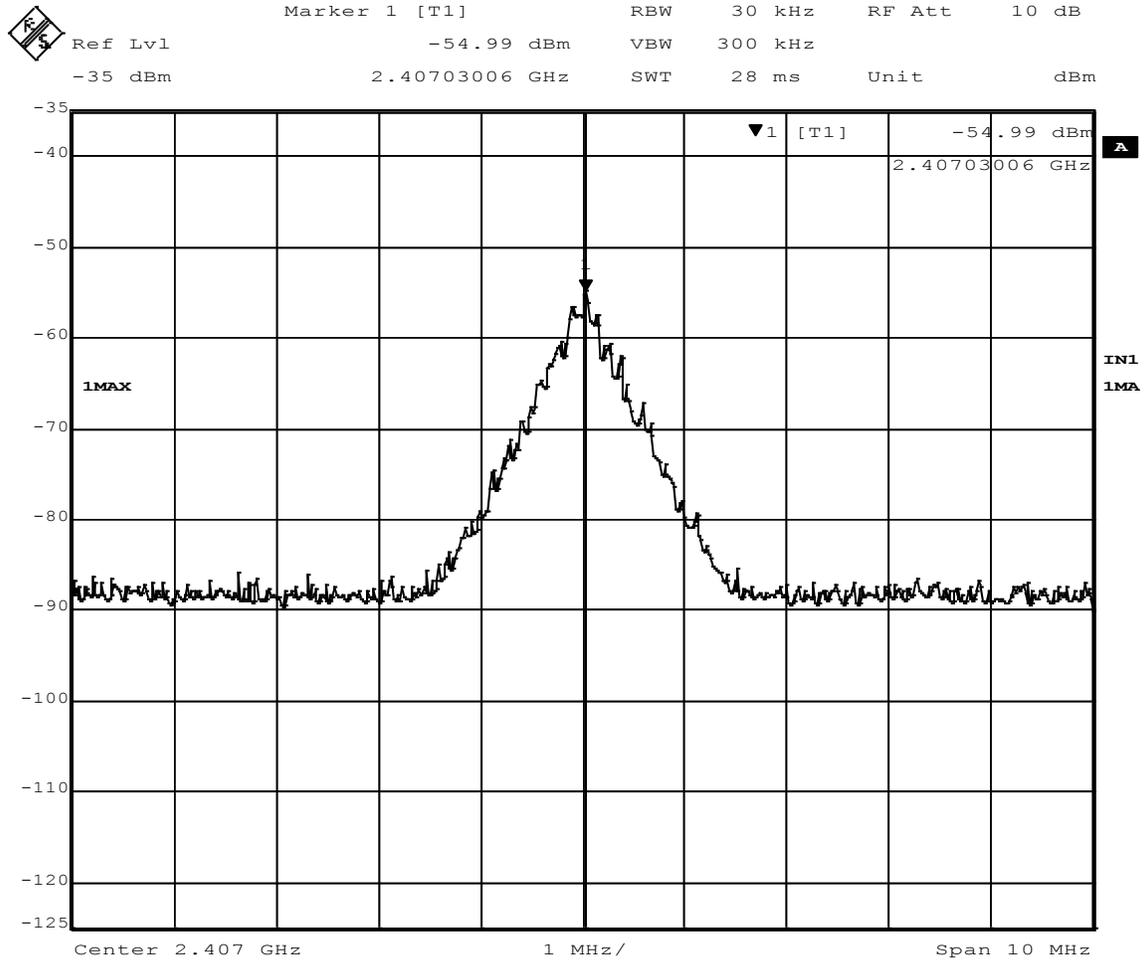
**Figure 14 - Band-edge Measurement, Low Channel, Fundamental**
