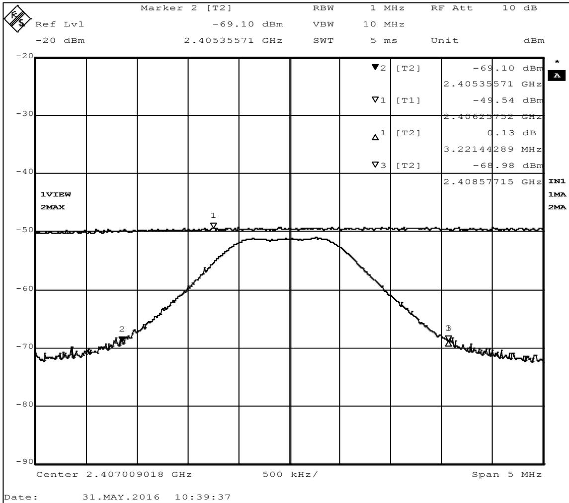
**Figure 10 - 99% Occupied Bandwidth, Low Channel. 3.22 MHz**
