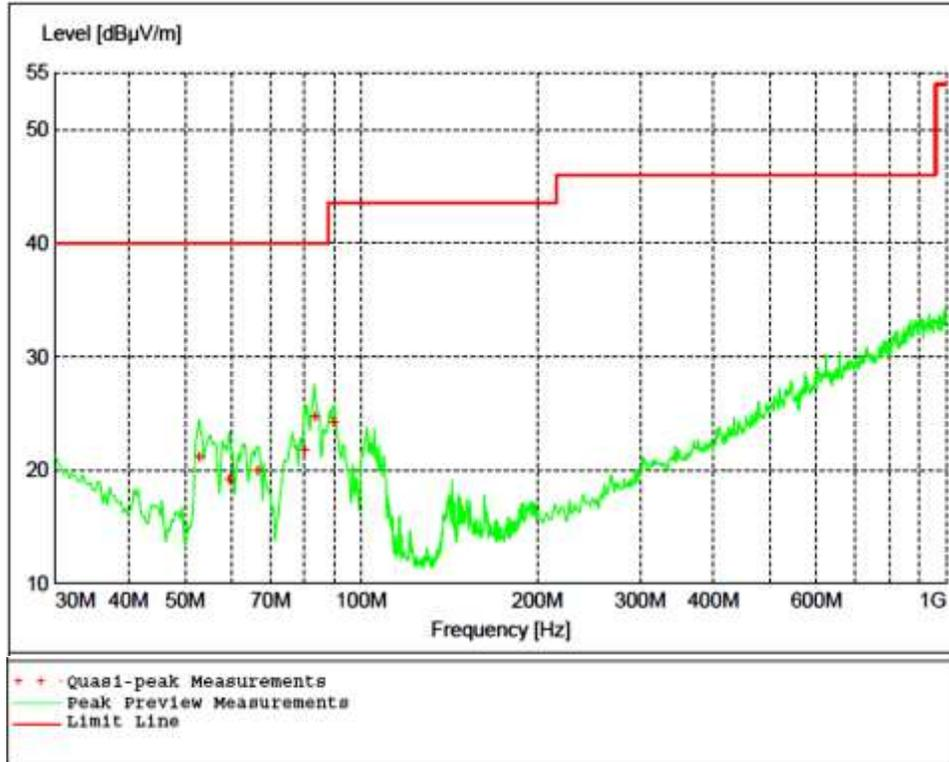
**Figure 4 - Radiated Emissions Plot, Mid Channel**
