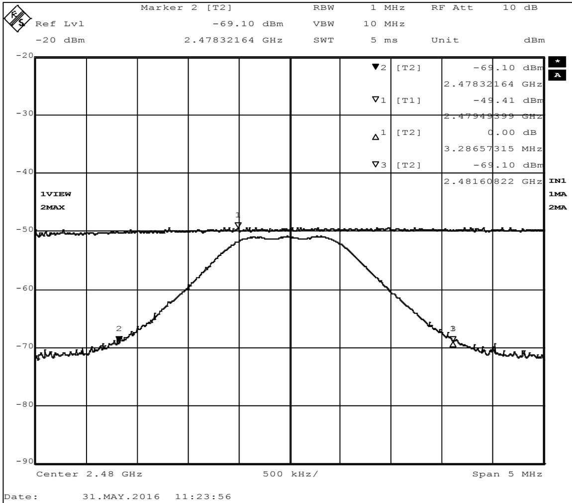
Figure 12 - 99% Occupied Bandwidth, High Channel, 3.28 MHz
