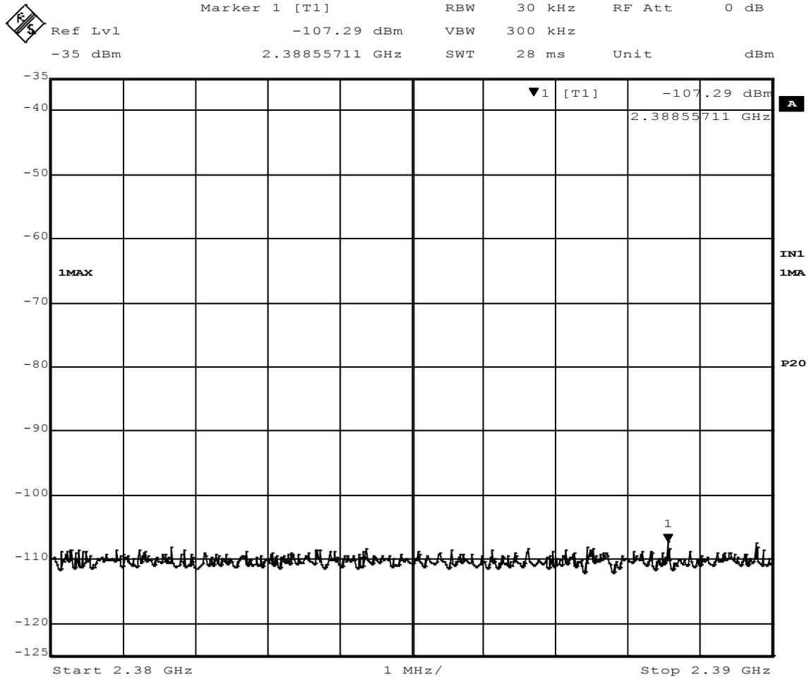
**Figure 13 - Band-edge Measurement, Low Channel, Restricted Frequency**
