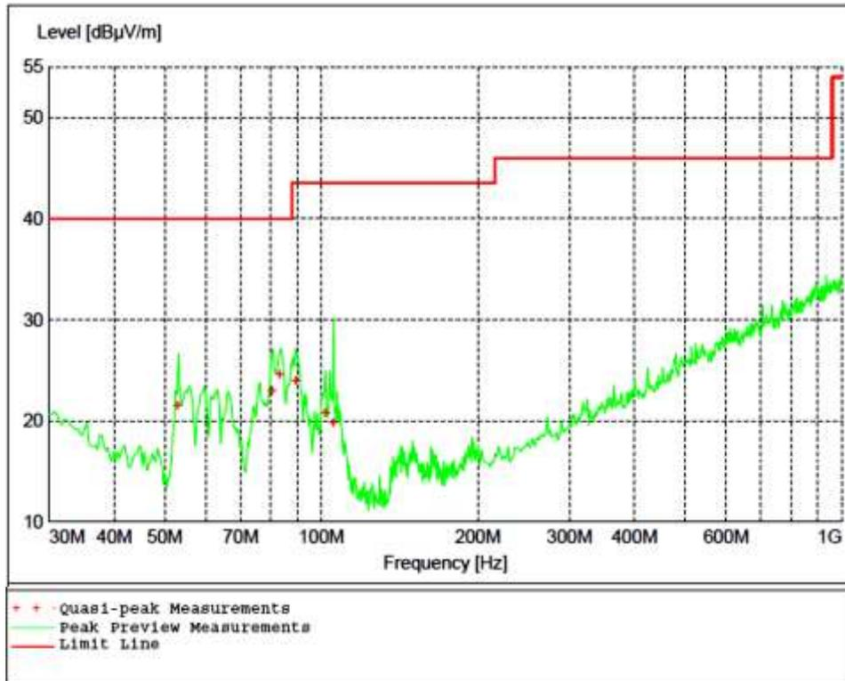
**Figure 3 - Radiated Emissions Plot, Low Channel**
