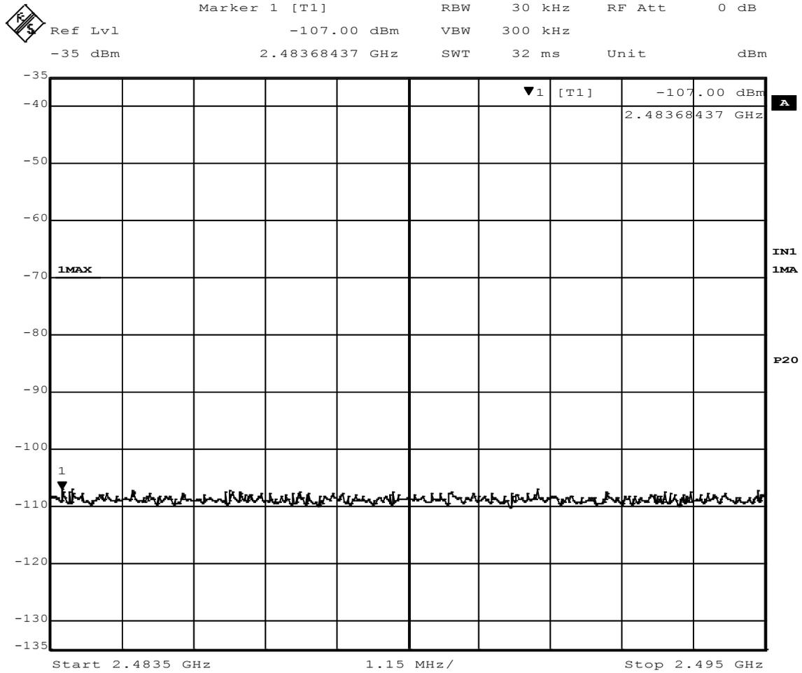
**Figure 15 - Band-edge Measurement, High Channel, Restricted Frequency**
