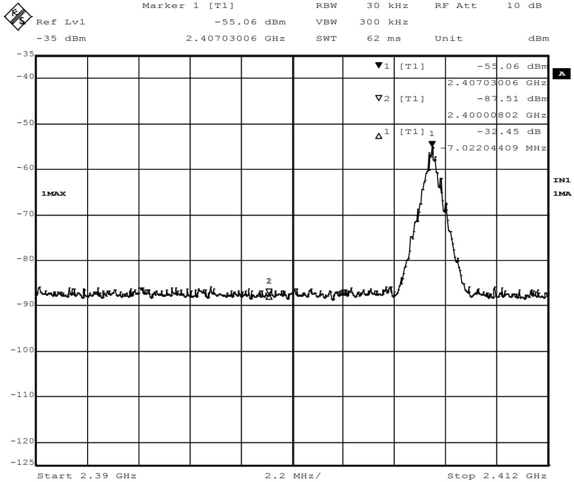
**Figure 17 – Band-edge Measurement, High Channel, out-of-band**
