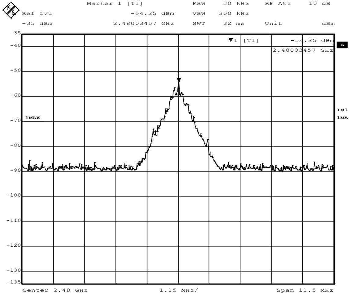
**Figure 16 - Band-edge Measurement, High Channel, Fundamental**
