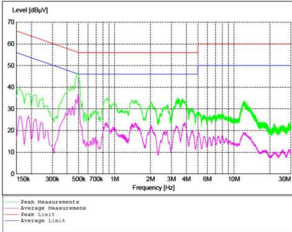
Figure 18 - Conducted Emissions Plot
