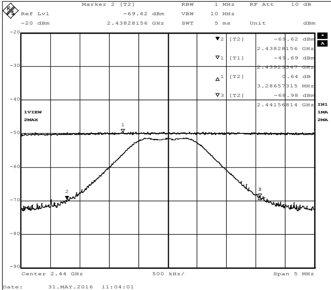
**Figure 11 - 99% Occupied Bandwidth, Mid Channel, 3.28 MHz**
