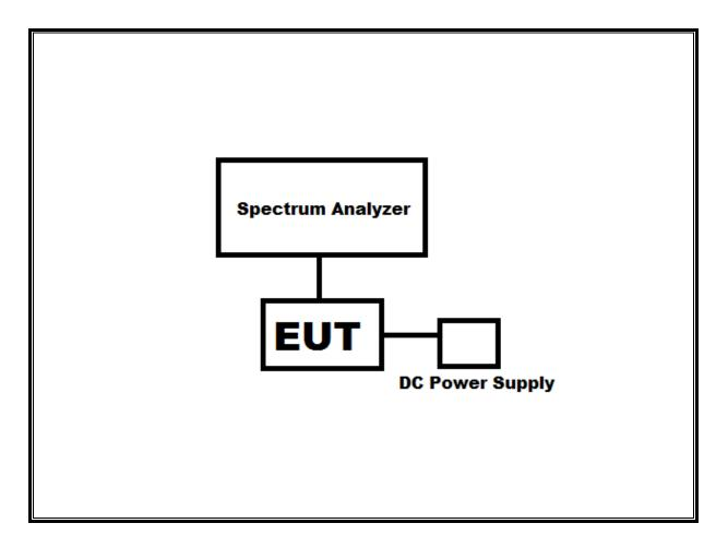
\*Note – The DC power supply is used only during testing. During normal operation the EUT is powered by a supplied battery pack
