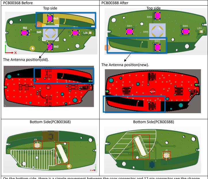
On the bottom side, there is a simple movement between the coax connector and 12 pin connector see the change, also removed one hole.
