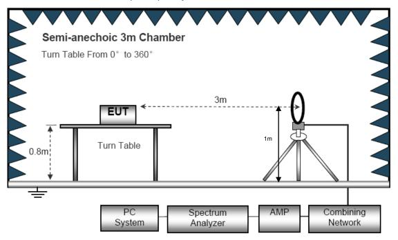
(B) Radiated Emission Test-Up Frequency 30MHz~1GHz
