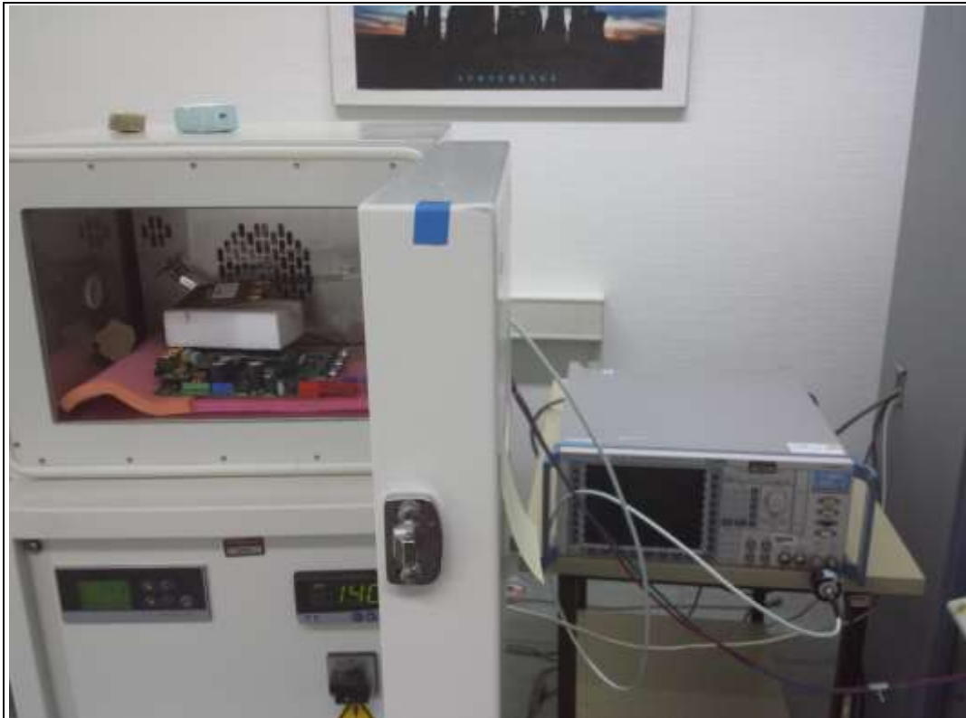
Photograph 1: Conducted measurements - Frequency error
