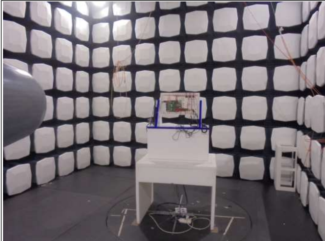
Photograph 5: Radiated mission measurements (overview)
