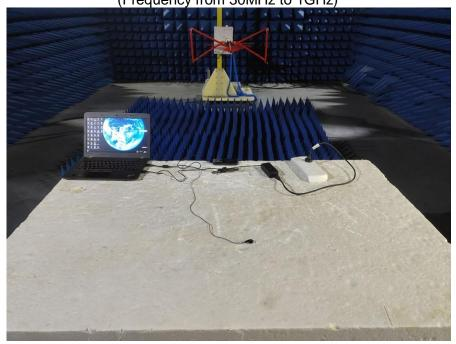
RADIATED EMISSION TEST (Frequency above 1GHz)
