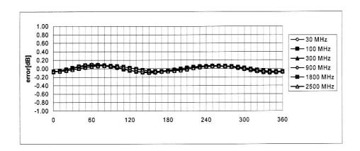
Axial Isotropy Error < ± 0.2 dB
