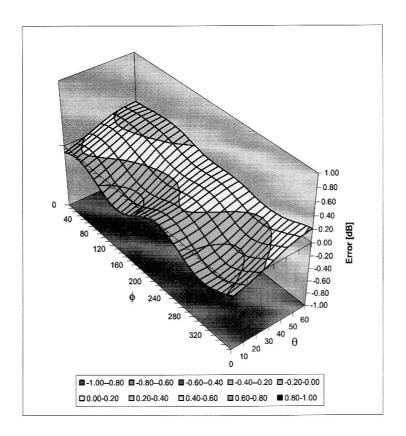
Spherical Isotropy Error < ± 0.4 dB
