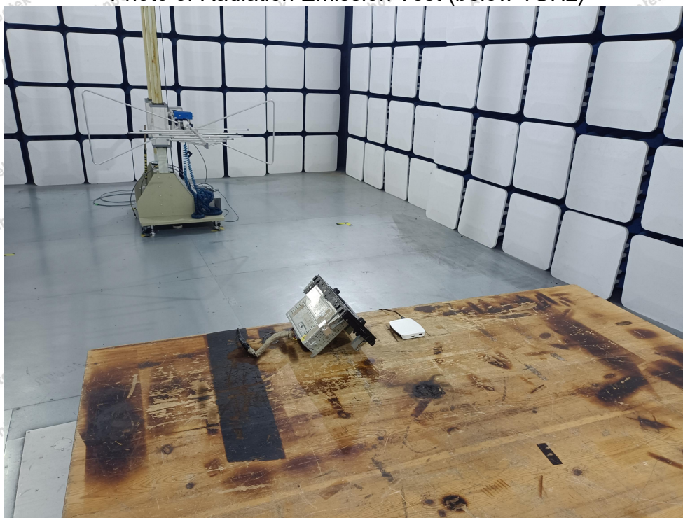
Photo of Radiation Emission Test (below 1GHz)
