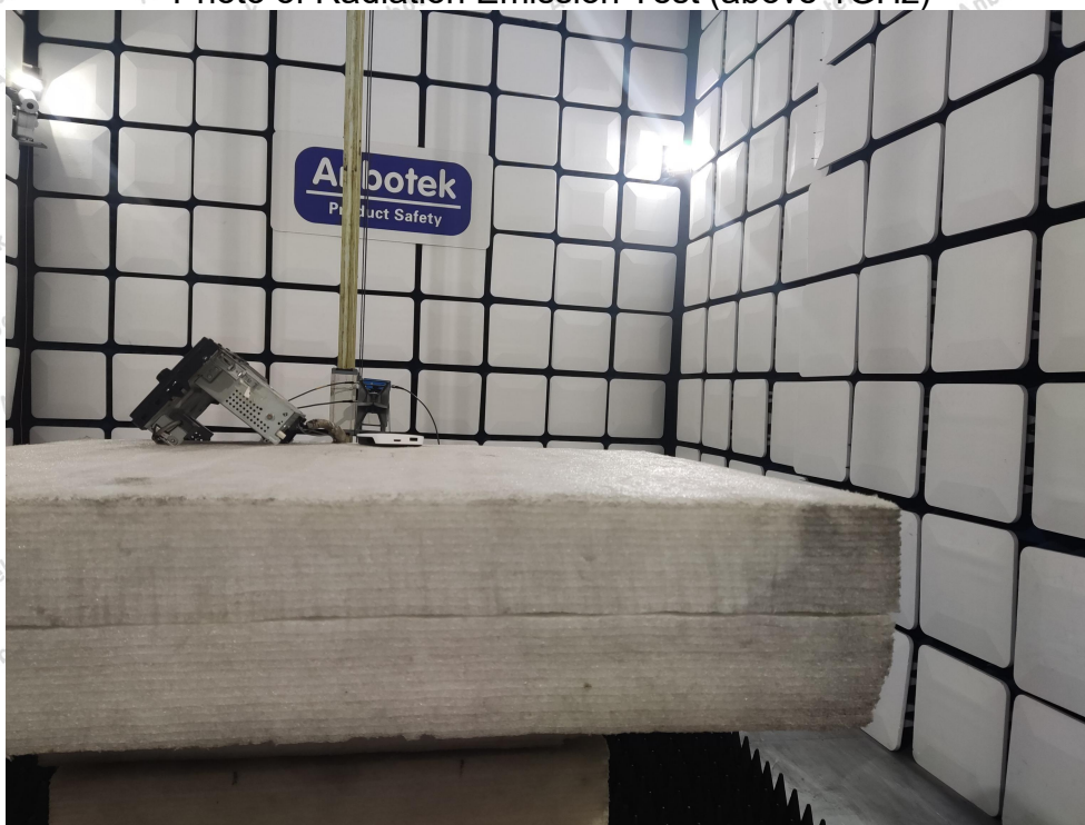
Photo of Radiation Emission Test (above 1GHz)
