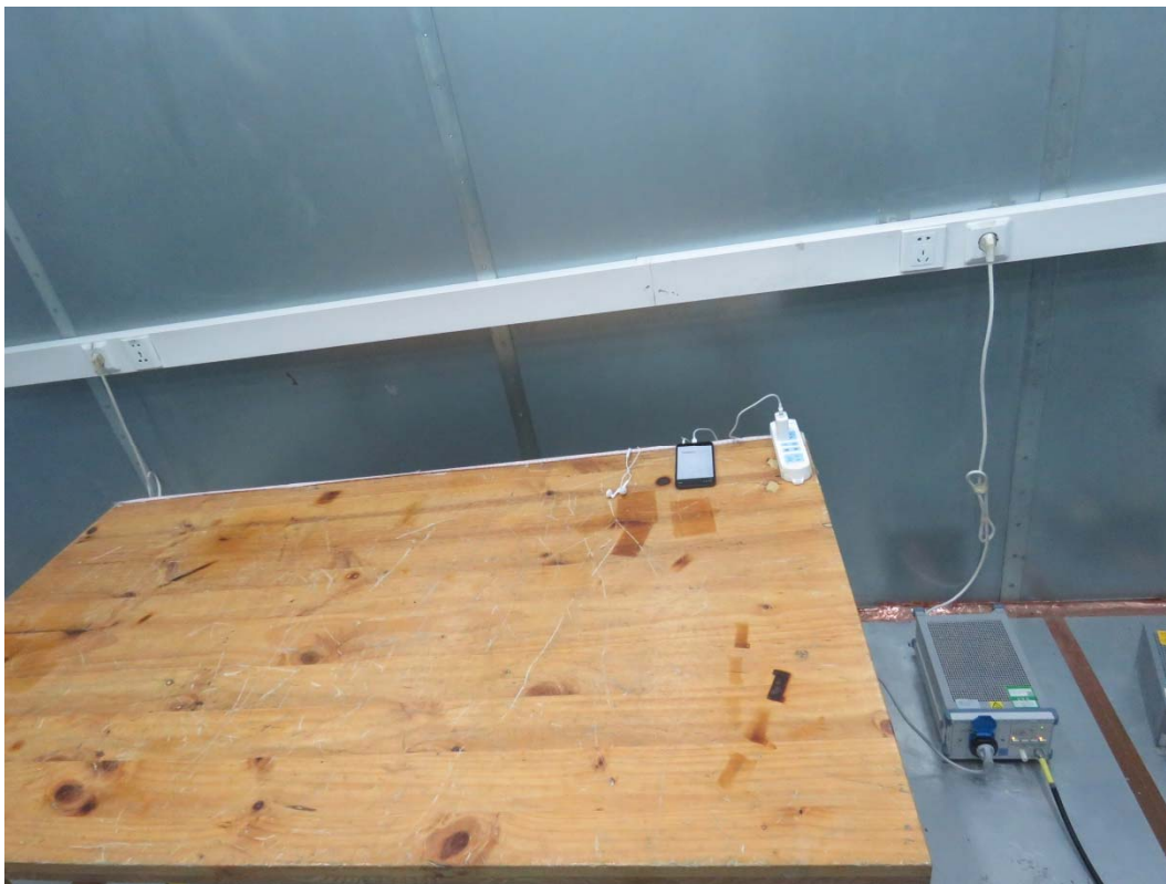
Picture 2 Conducted Emission Test Setup
