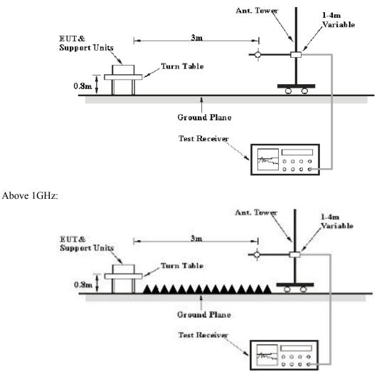
The radiated emission tests were performed in the 3 meters chamber, using the setup accordance with the ANSI C63.4-2014. The specification used was with the FCC Part 15 B Class B limits.
