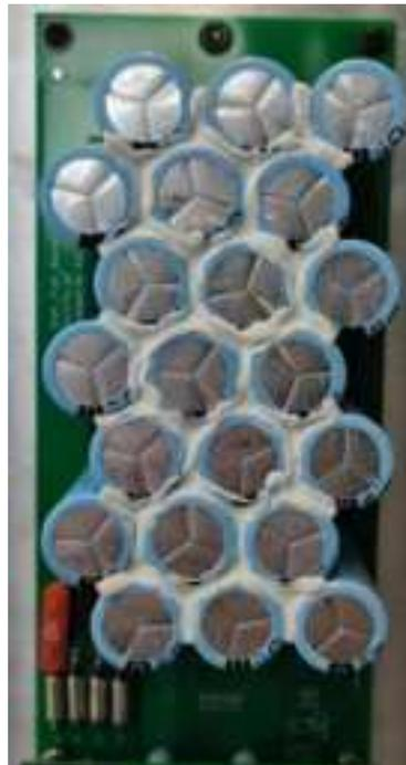
Figure 2. Super Capacitor Board
