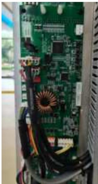
Figure 3. Power Control Board
