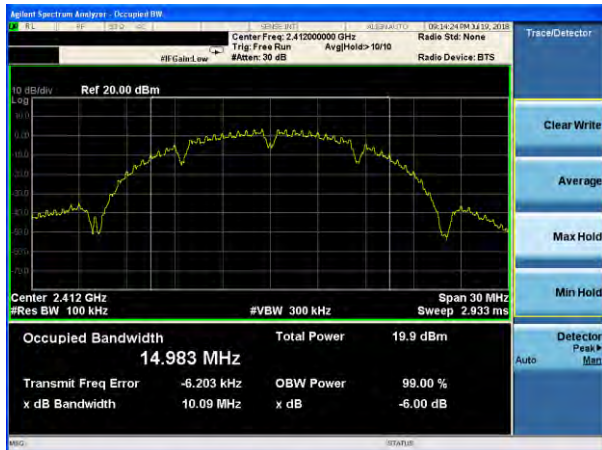
(802.11b) 6dB Bandwidth plot on channel 6
