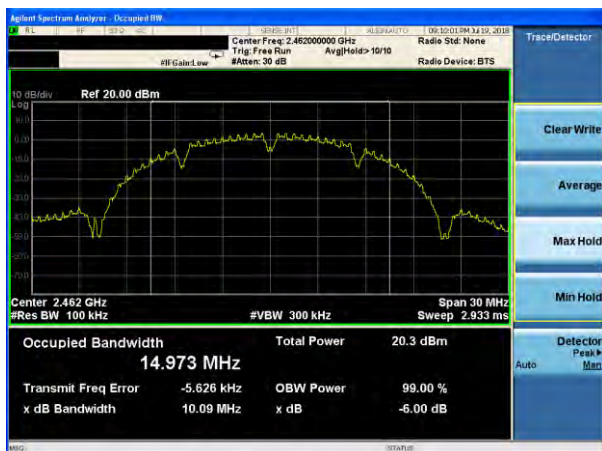
(802.11b) 6dB Bandwidth plot on channel 11
