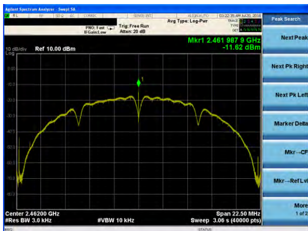
(802.11b) PSD plot on channel 11
