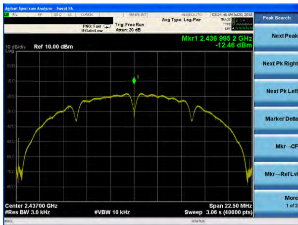
(802.11b) PSD plot on channel 6
