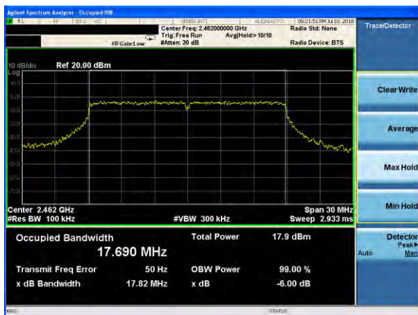
(802.11n20) 6dB Bandwidth plot on channel 11
