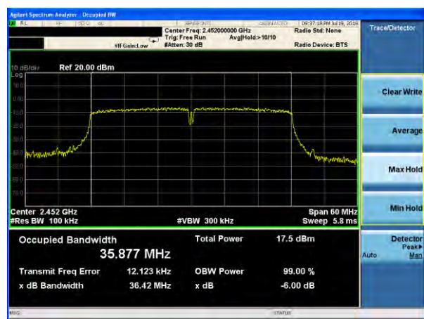
(802.11n40) 6dB Bandwidth plot on channel 9
