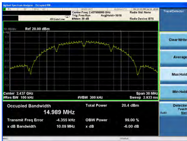
(802.11b) 6dB Bandwidth plot on channel 11
