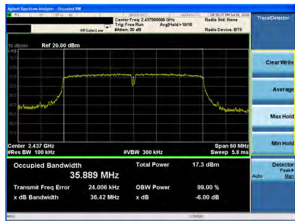
(802.11n40) 6dB Bandwidth plot on channel 6
