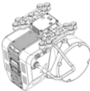
**Data cable connection:** unplug the dust cap (round silver metal cap) of the data interface on the side of the scanner body, and pay attention to aligning the red dot mark at the data cable interface of the bracket with the red dot mark of the data interface of the body before insert link;
