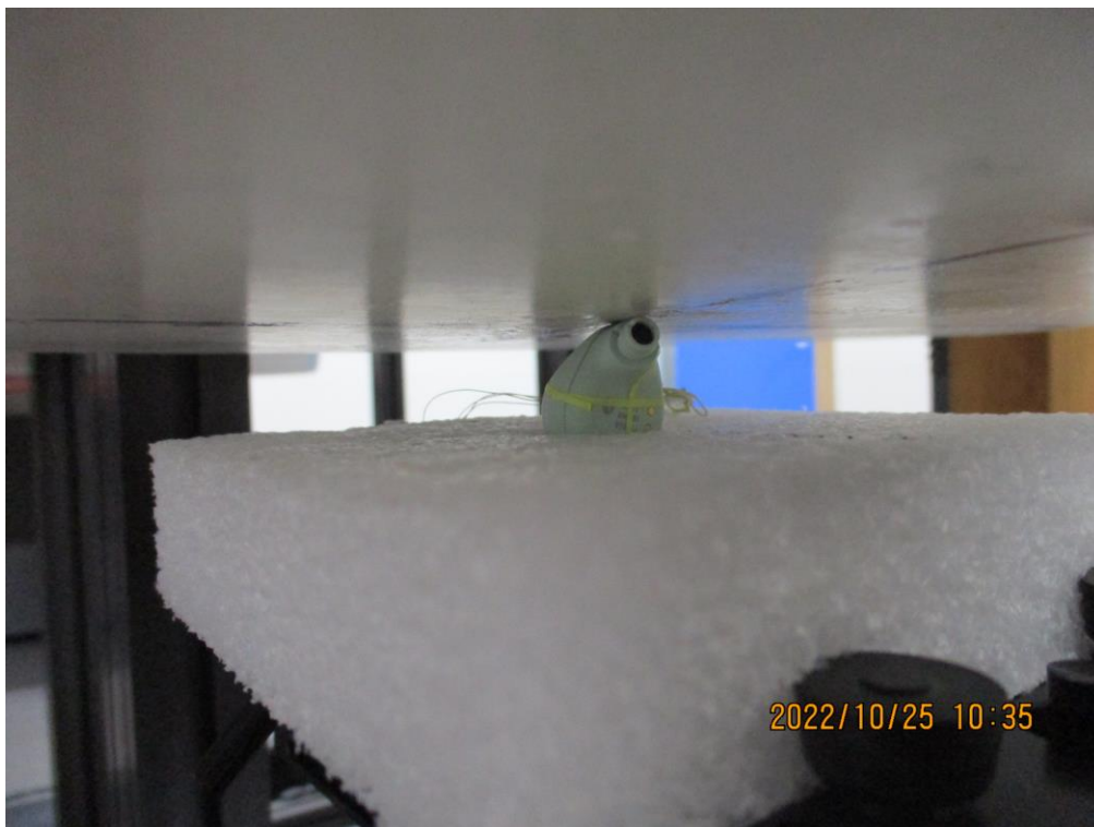
Bottom from Flat Phantom (Separation Distance: 0 cm) – Left Ear
