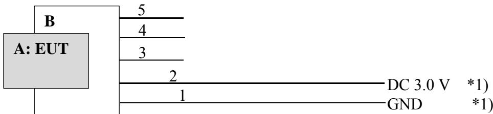
\*1) DC power supply (Model No.: PAN55-20A) was used for DC 3.0 V / GND input.
