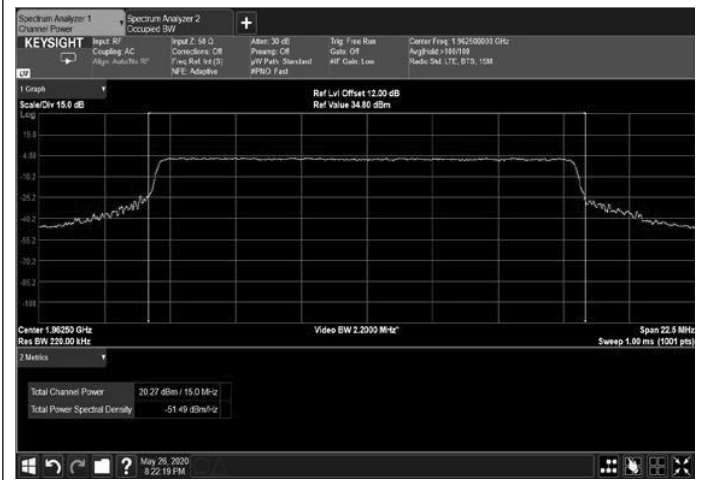
Figure 58: 64QAM 15MHz B.W.; 1962.5MHz, 15Hz
