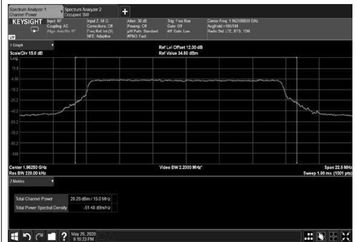
Figure 60: 64QAM 15MHz B.W.; 1962.5MHz, 60Hz
