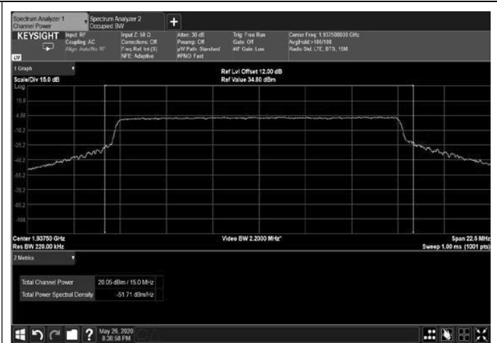
Figure 56: 64QAM 15MHz B.W.; 1937.5MHz, 30Hz
