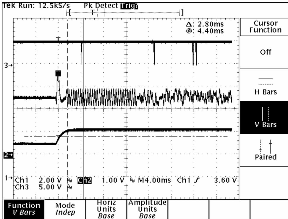
The recovered modulation should be centered at approximately 2.5 VDC and should have an amplitude of approximately 800 mV peak-to-peak as indicated in the plot above.
