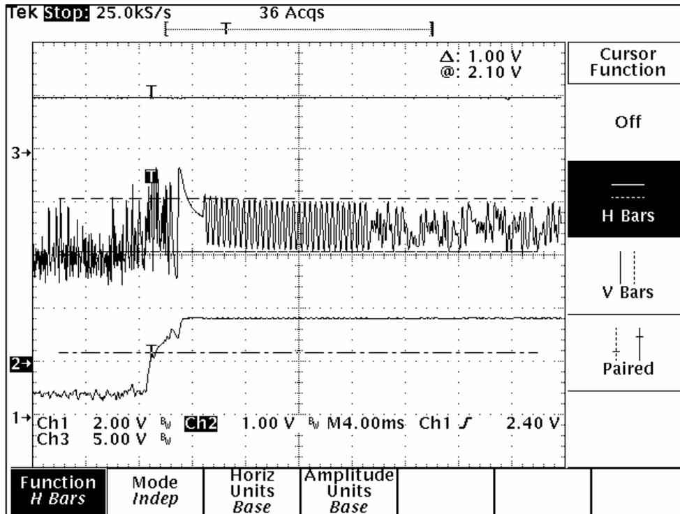
As seen in the above plot, the mobile radio's transmit carrier has ramped up to full power (channel 1) in just a few milliseconds. The recovered modulation (channel 2) is stable by this time. There follows a few milliseconds of quiet time followed by 12 milliseconds of symbol sync time.
