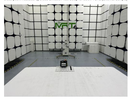
Description: Radiated Spurious Emission Test Setup for above 1GHz (External Sample)
