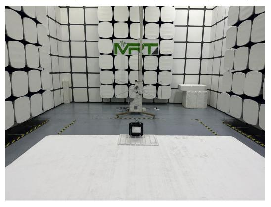
Description: Radiated Spurious Emission Test Setup for above 1GHz (Internal Sample)
