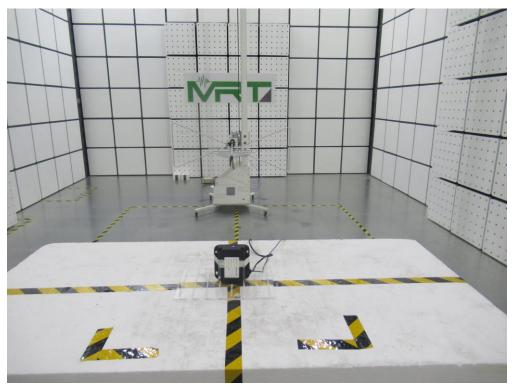
Description: Radiated Spurious Emission Test Setup for above 1GHz (Internal Sample)
