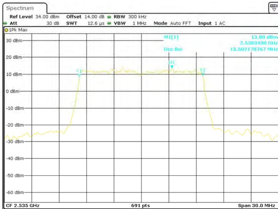
**QPSK (15.0 MHz) - 26 dB Bandwidth, Middle channel**
