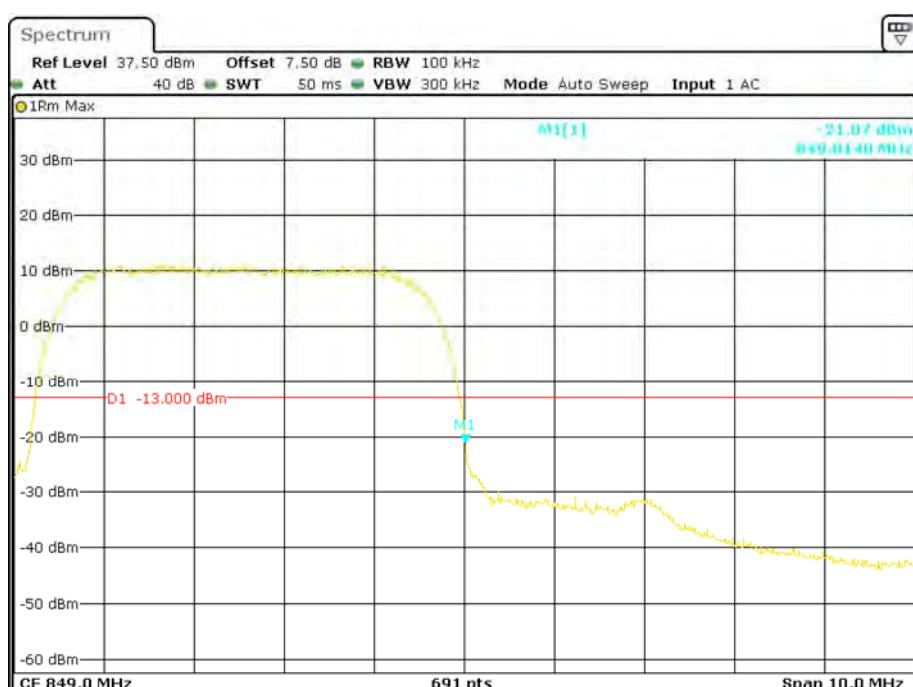
**Cellular Band, Left Band Edge for HSDPA (16QAM) Mode**
