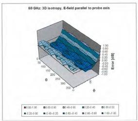
Probe isotropy for  $E_{tot}$ : probe rotated  $\phi = 0^{\circ}$  to 360°, tilted from field propagation direction  $\vec{k}$ Parallel to the field propagation ( $\psi$  =0° - 90°) at 30 GHz: deviation within ± 0.46 dB Parallel to the field propagation ( $\psi$  =0° - 90°) at 60 GHz: deviation within ± 0.44 dB
