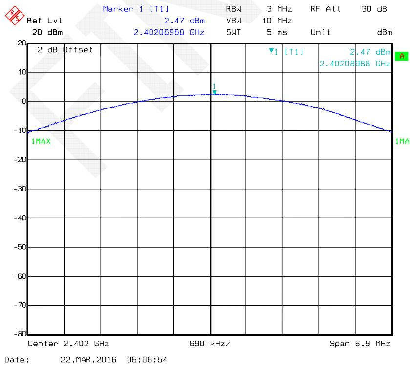
**Output Power, Middle Channel**
