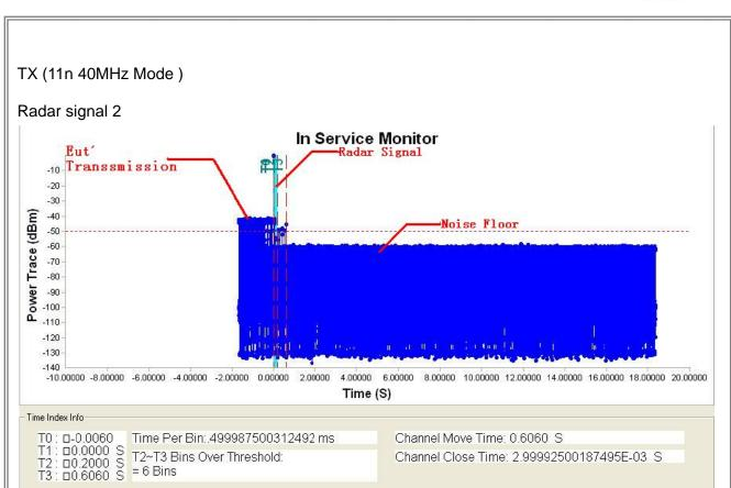
**Note:** To denotes the start of Channel Move Time upon the end of the last Radar burst.
