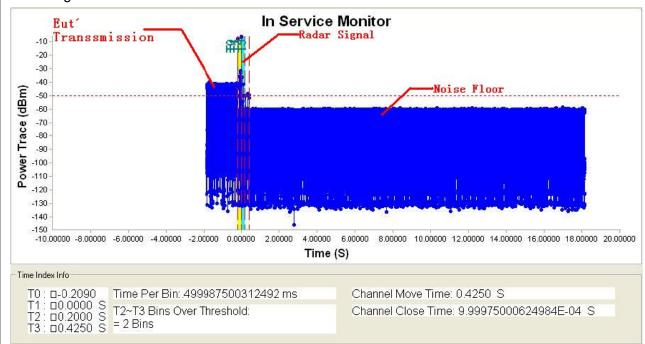
Note: T0 denotes the start of Channel Move Time upon the end of the last Radar burst.
