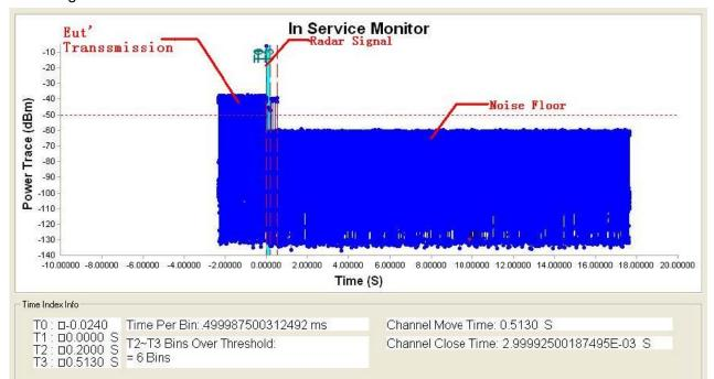
**Note:** To denotes the start of Channel Move Time upon the end of the last Radar burst.
