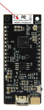
The label shown shall be permanently affixed at a conspicuous location on the device and be readily visible to the user at the time purchase (Labeling requirements per 2.925)
