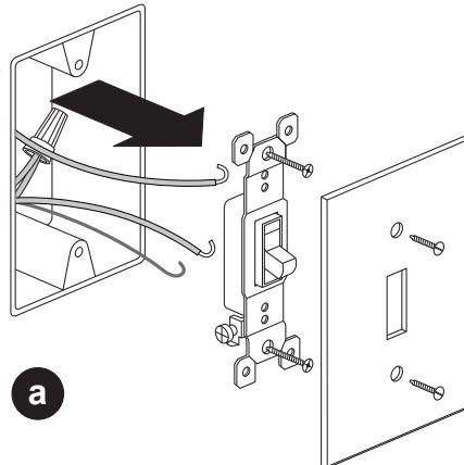
In case of multi-gang installation, replace the provided frame with adorne™ multi gang frame.
