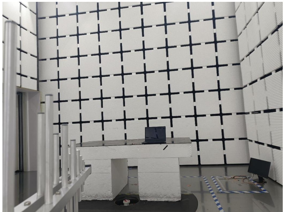
Radiation Emission Test Setup (30MHz to 1GHz)
