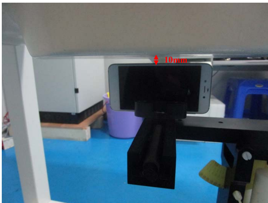
Body-worn Left Setup Photo
