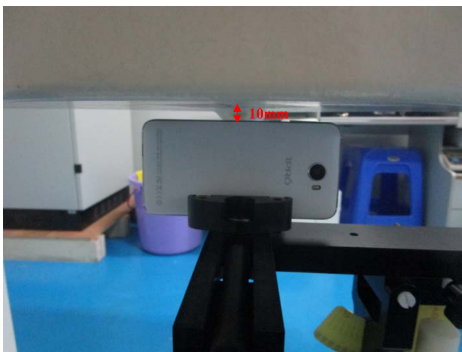
Body-worn Right Setup Photo
