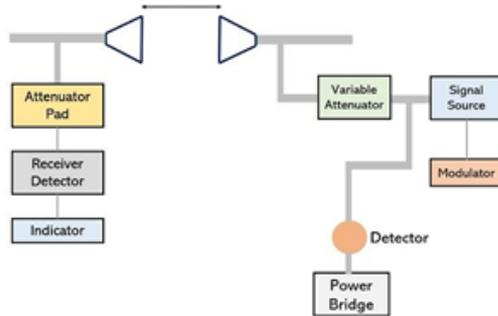
Suppose the two antennas (transmitting and receiving) are separated at a distance  $r$ . Here,  $P_t$  and  $P_r$  represent the transmitted and received power respectively. While  $A_{et}$  and  $A_{er}$  are the effective apertures of transmitting and receiving antennas.
