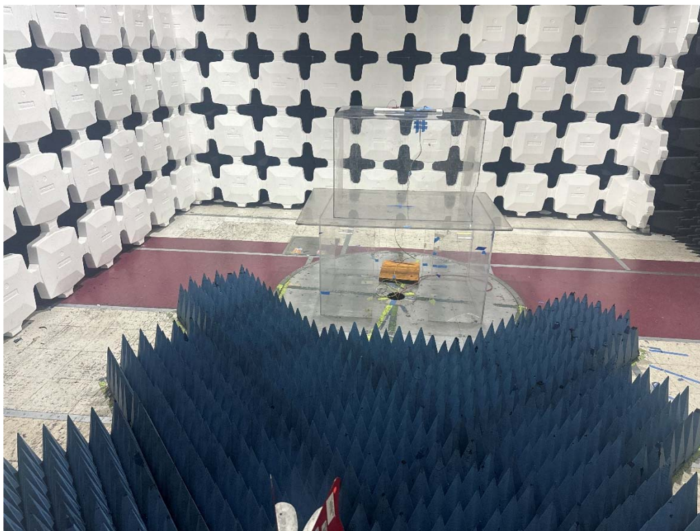
Radiated Emission Test above 1GHz Front View
