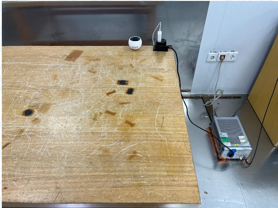
Photo of Setup for Radiated Emission (30MHz~1GHz)
