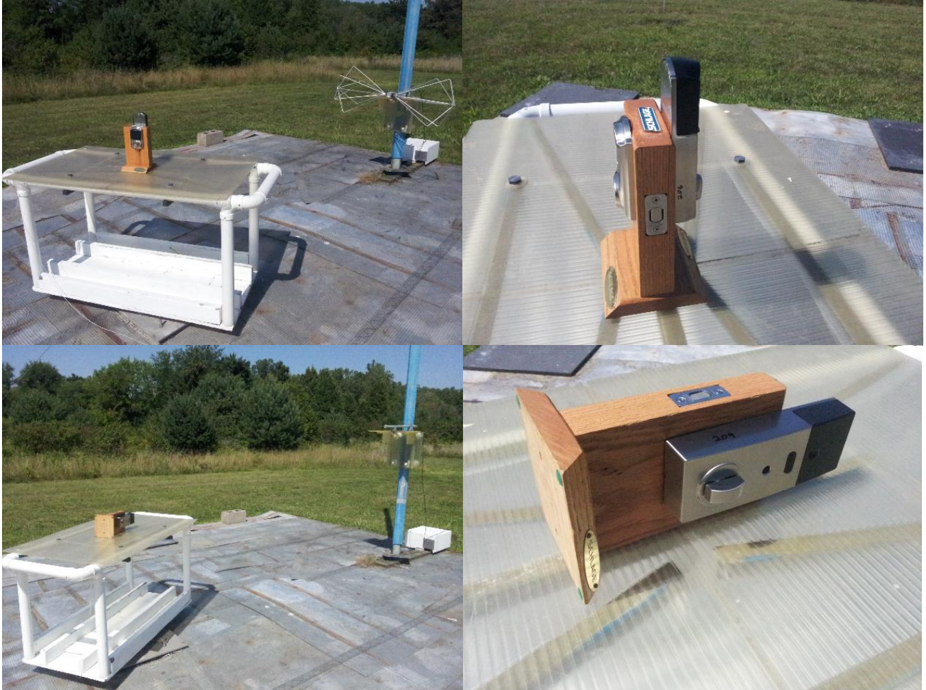
Figure 4: Radiated Emissions Test Setup Photograph(s).
