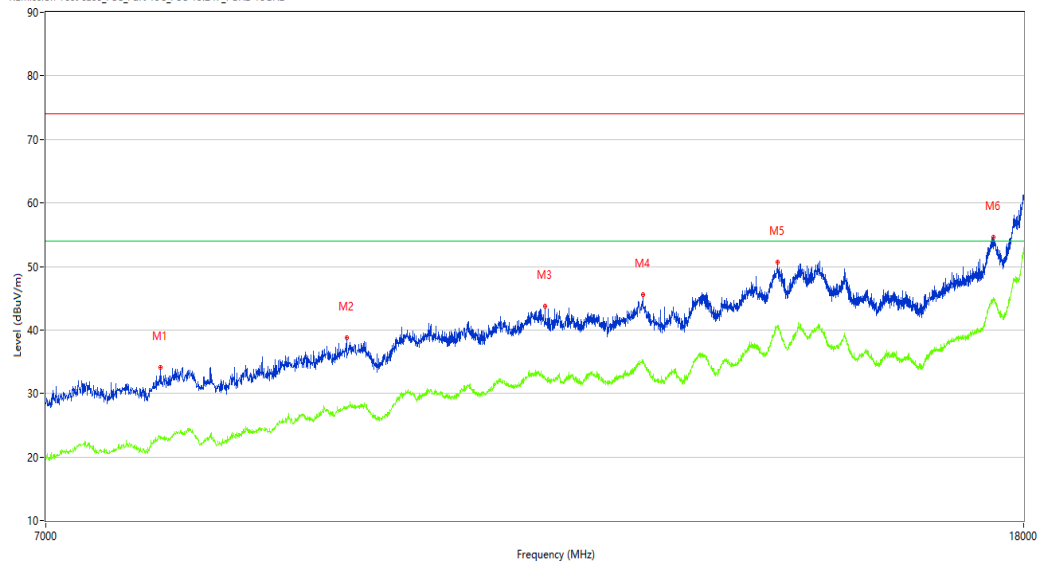
REmission Test case_FCC_Part 15C_FCC 15.247_7GHz-18GHz
