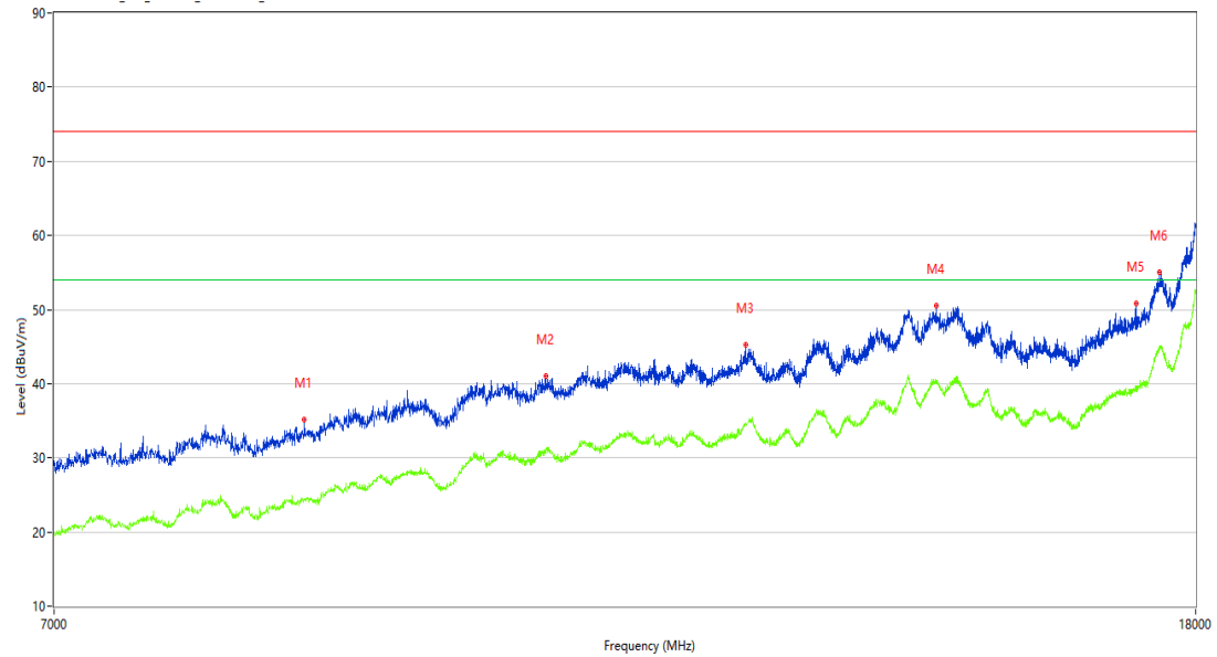
REmission Test case_FCC_Part 15C_FCC 15.247.7GHz-18GHz
