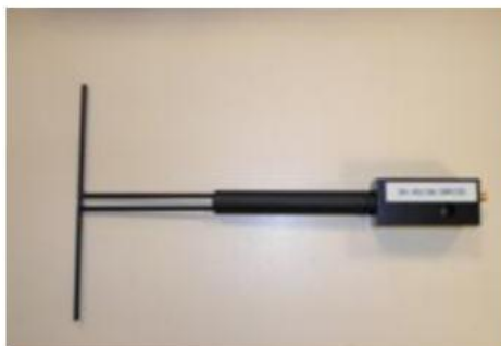
Figure 1 – Satimo COMOSAR Validation Dipole
