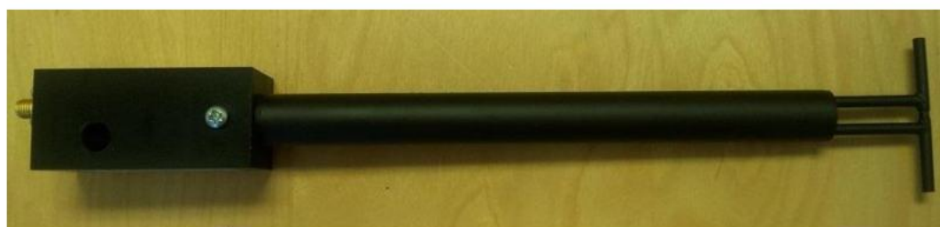
Figure 1 – MVG COMOSAR Validation Dipole
