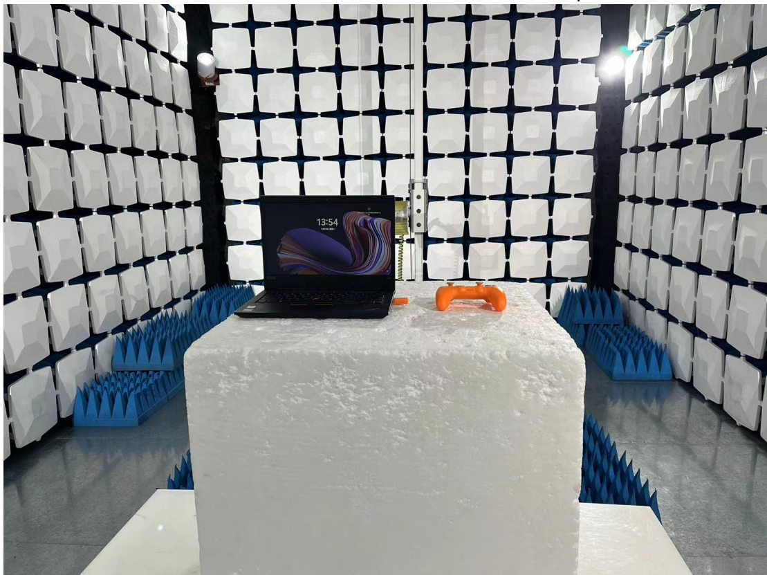
Above 1GHz for radiated emission test setup
