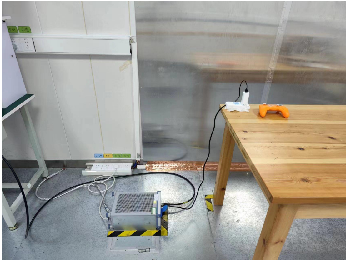
Conducted emission test setup
