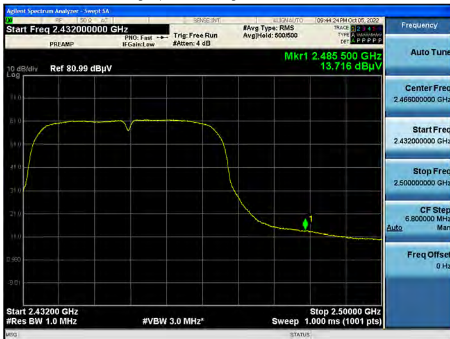
Radiated Restricted Band Edges plot – Average Result (802.11n (HT40), Ch.9(2 485.5 MHz))
