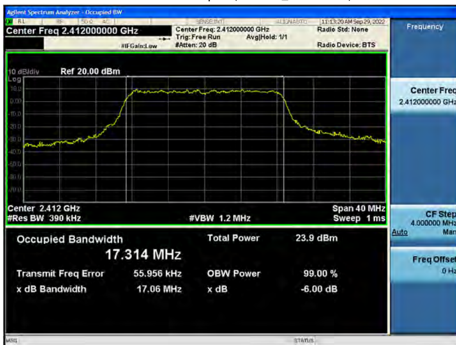
99 % Bandwidth plot (802.11n_HT20-CH 1)
