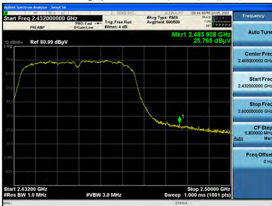
Radiated Restricted Band Edges plot – Peak Result (802.11n (HT40), Ch.9(2 483.5 MHz))
