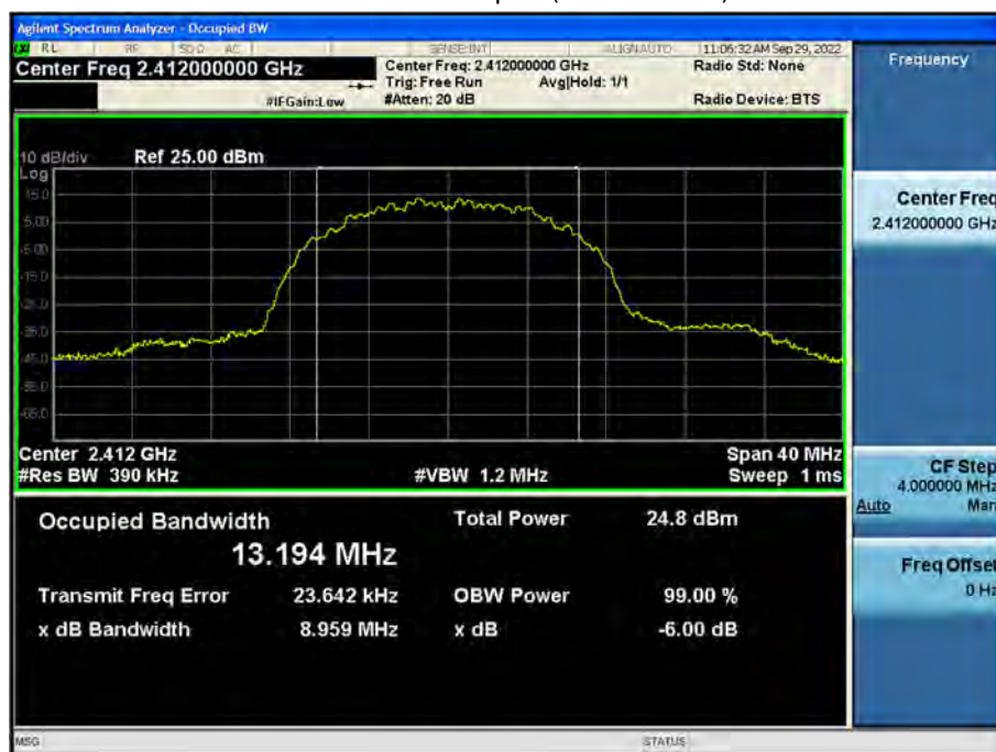
99 % Bandwidth plot (802.11b-CH 1)
