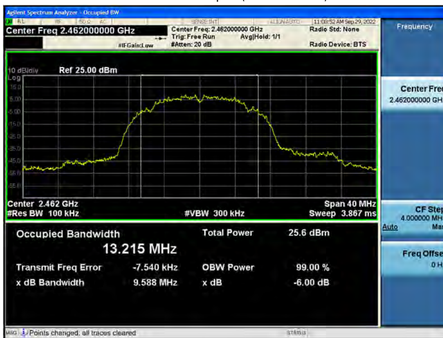
6 dB Bandwidth plot (802.11b-CH 11)
