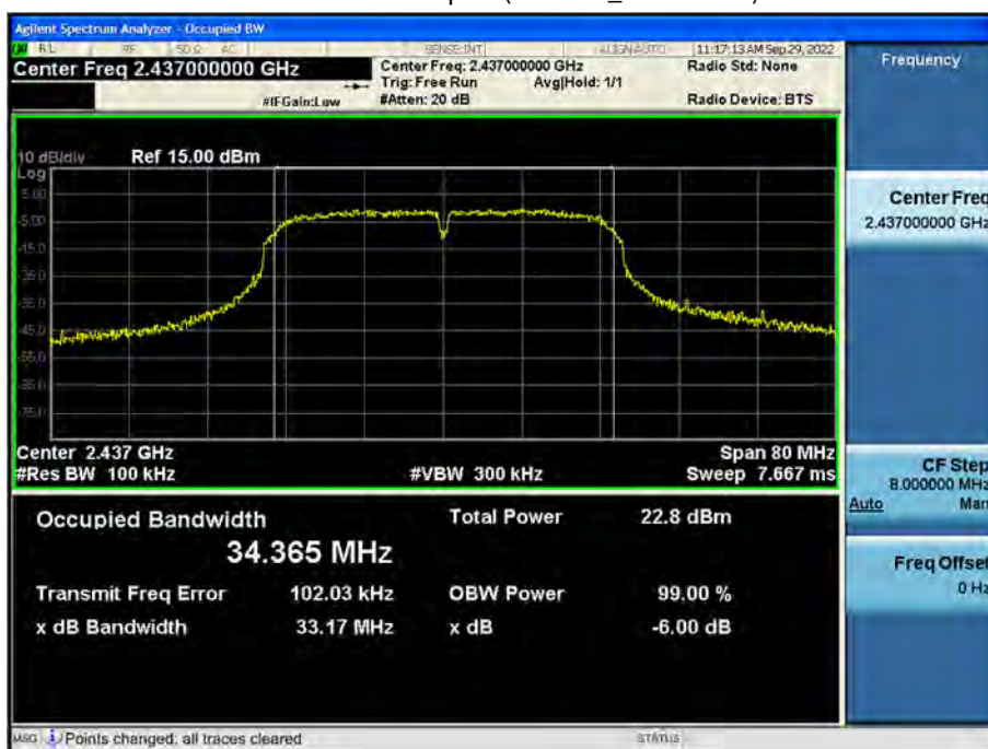
6 dB Bandwidth plot (802.11n_HT40-CH 6)
