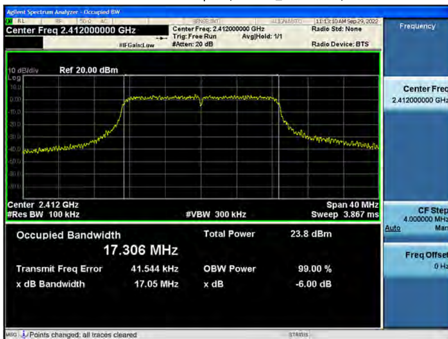
6 dB Bandwidth plot (802.11n_HT20-CH 1)
