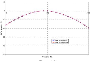
Figure 4-9 ABM2 Frequency Response Validation
