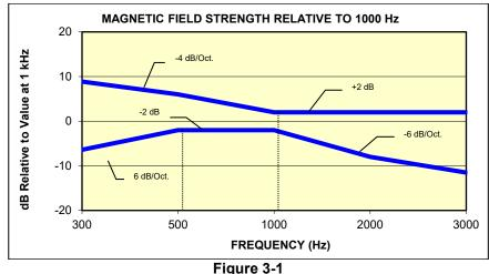
Magnetic field frequency response for Wireless Devices with an axial field ≤-15 dB(A/m) at 1 kHz
