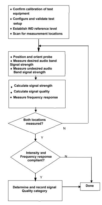
Figure 4-15 C63.19 T-Coil Signal Test Process
