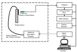
Figure 4-14 Audio Magnetic Field Test Setup
