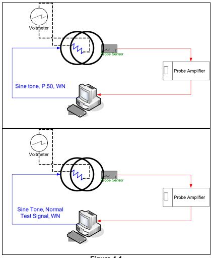
Figure 4-1 Validation Setup with Helmholtz Coil
