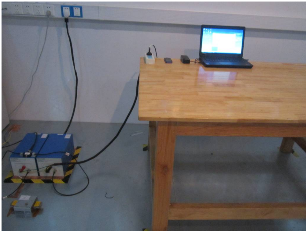
Conducted Emissions Test Setup Front View
