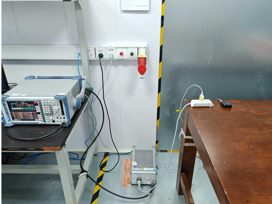
Conducted emissions at AC power line (150kHz-30MHz)
